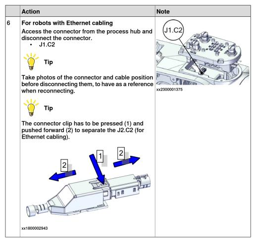
Disconnecting the axis-4 motor connectors
