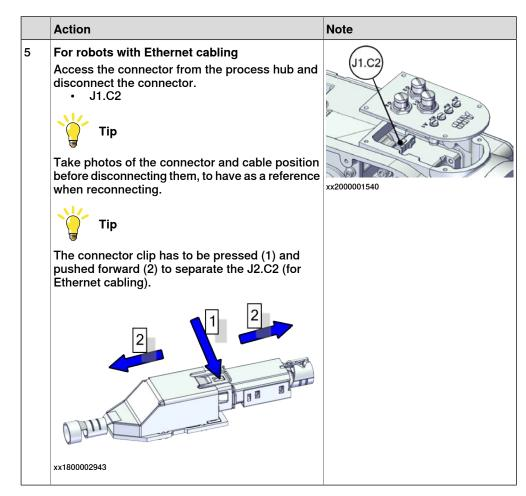
Removing the process hub (with solenoid valve)
