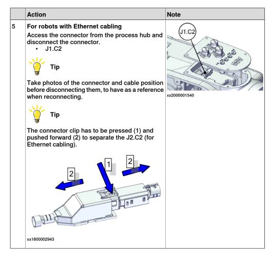
Removing the process hub (with solenoid valve)
