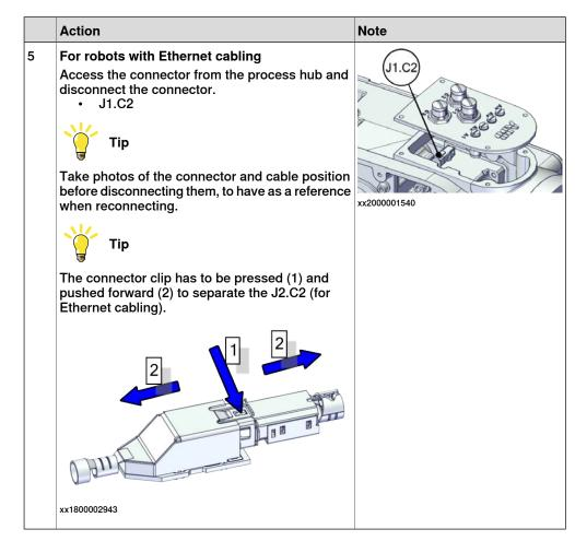
Removing the process hub (with solenoid valve)
