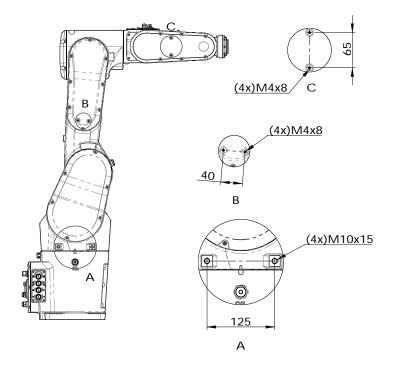
3.3.6 Fitting equipment on the robot (robot dimensions) *Continued*
