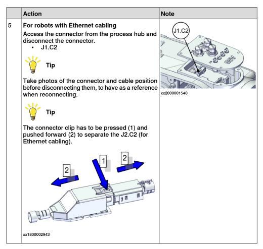
Removing the process hub (with solenoid valve)
