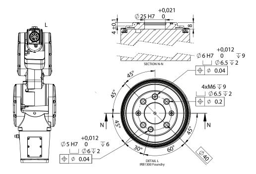
3.3.6 Fitting equipment on the robot (robot dimensions) *Continued*
